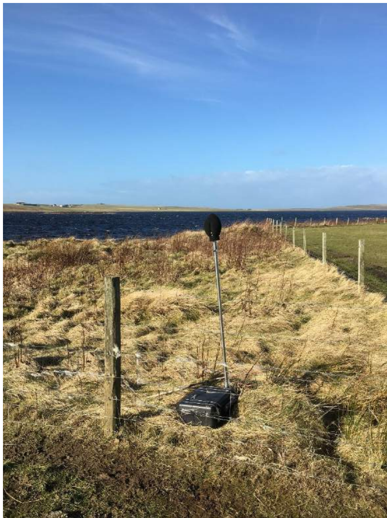
Photographs of SLM in position & identified noise sources
